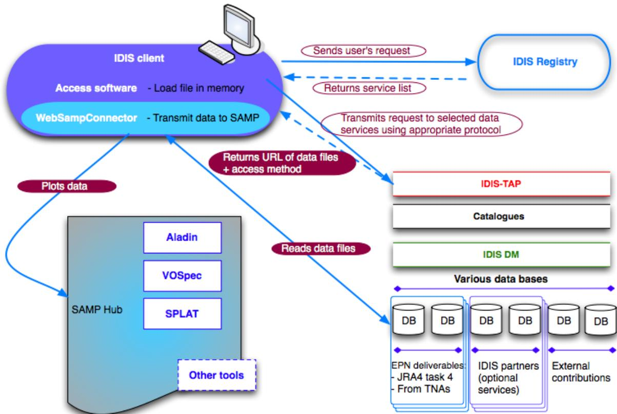
Figure 4: Overall data access through IDIS client
